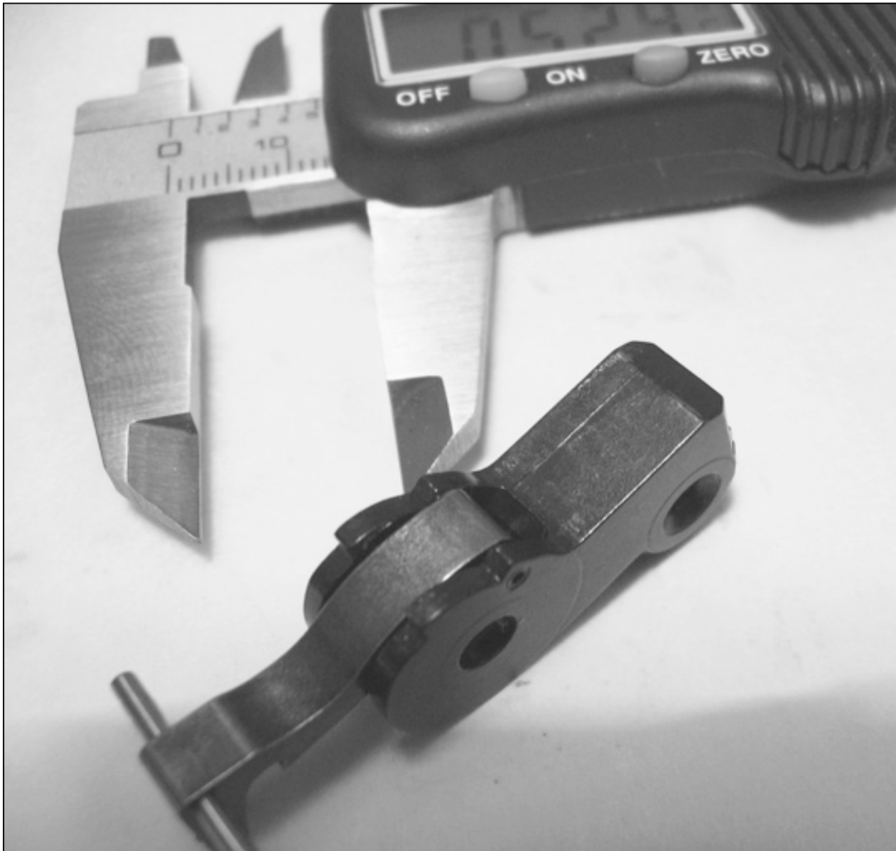
New style hammer ready for re-profiling.
