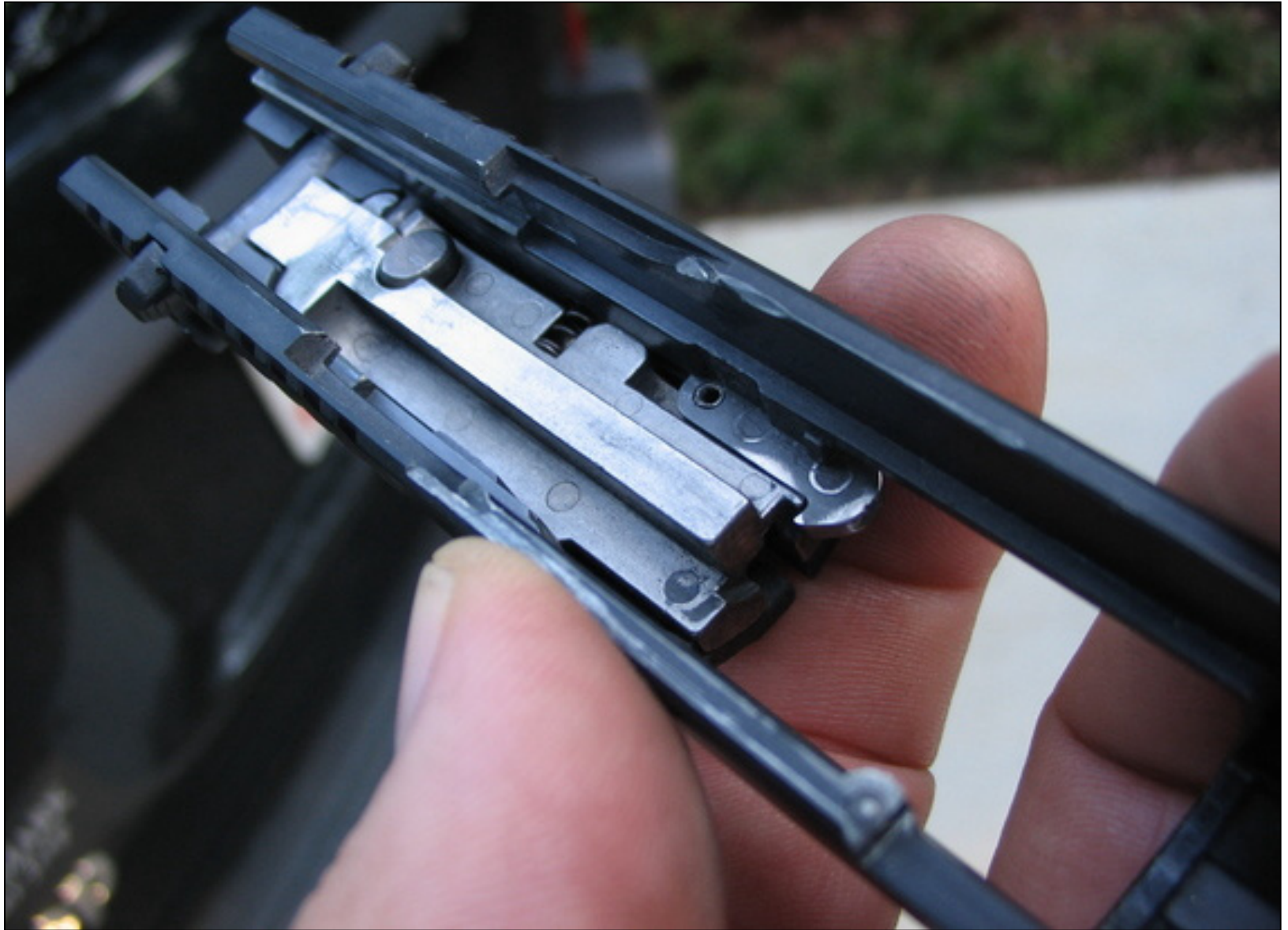
Extractor pin reinstalled and seated flush.
